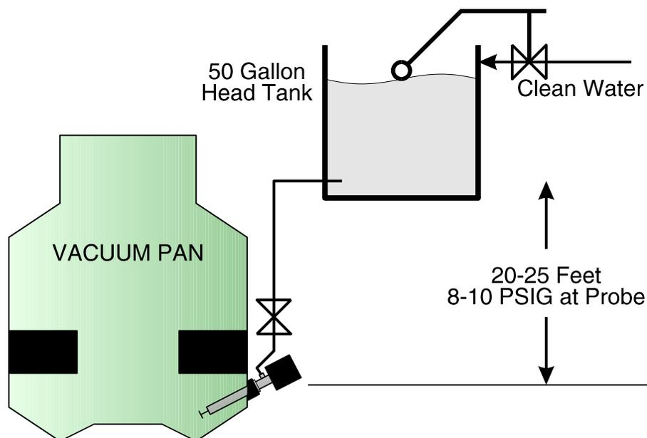
If water supply fails, turn off power to all operating probes until it is restored to prevent bearing and shaft damage. Adequately lubricated and purged bearings will not show excessive wear for over one year running time. Worn bearings are easily replaced. A spare set of bearings with mounting O-rings is furnished. See section titled "Bearing Replacement".
