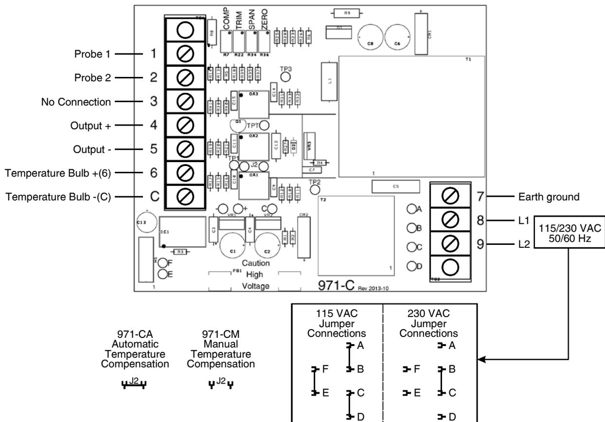
If the instrument was ordered as a 971-CM for manual temperature compensation, jumper J2 on the circuit board should not be installed (see Figure 5). On a 971-CA using a temperature compensating bulb, J2 should be installed and the bulb should be installed in the syrup near the probe rotor through a 3/4" NPT connection. Wires from the bulb connect to terminals C(-) and 6(+) as shown in Figure 5.
