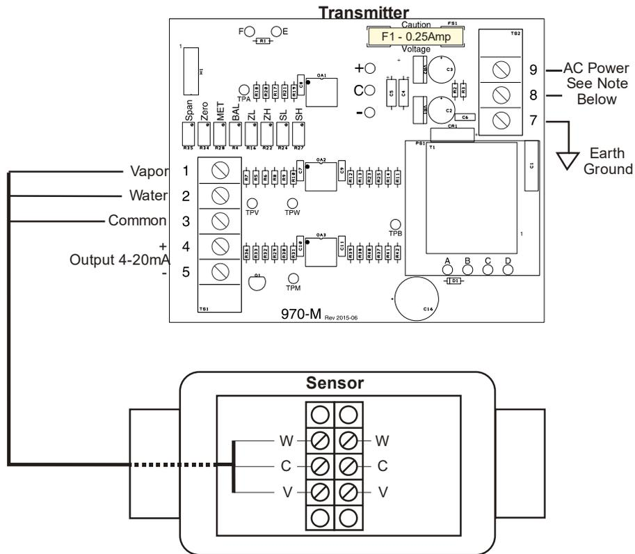
Transmitter Output: 4-20mA, 600 Ohms Max
