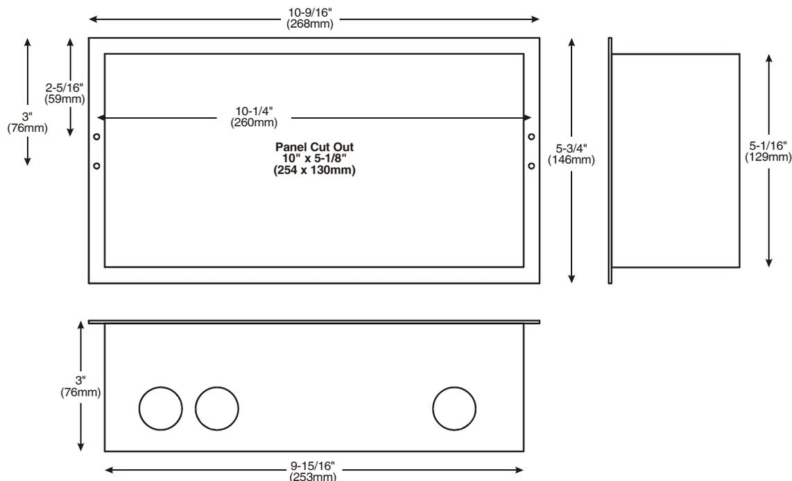
**Figure 3: NEMA 4X Enclosure Dimensions**
